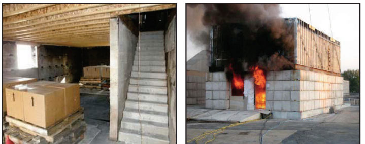
Figure 3: Field experiment townhouse test structures.
