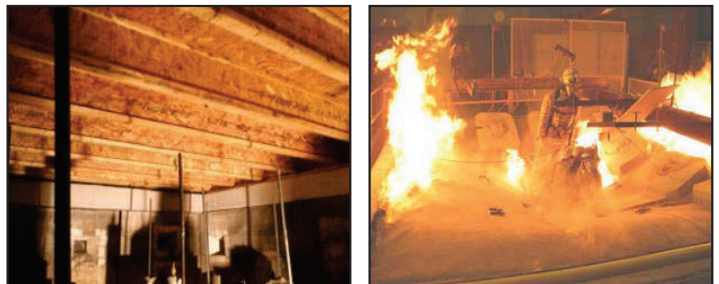
Figure 2: ASTM E119 floor furnace experiments with modified applied structural loads.
